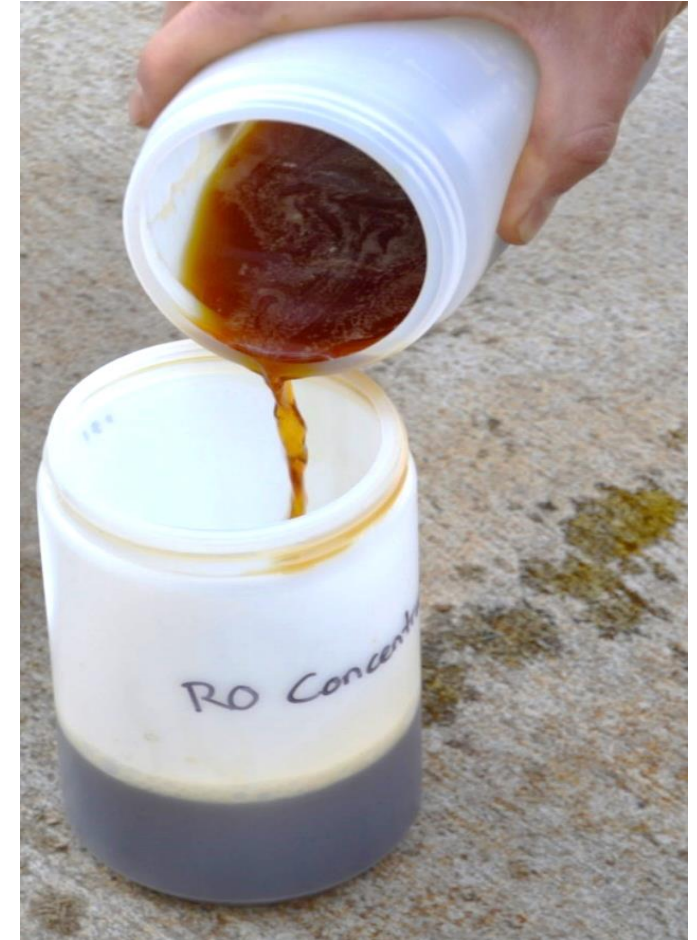
RO produces "RO Concentrate", a fertilizer rich in potassium and ammonia nitrogen.
