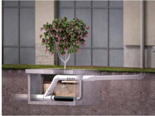
Filterra Internal Bypass-Pipe
